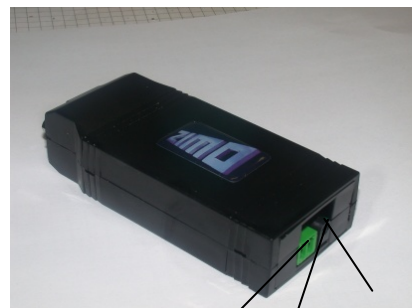
Connect to "update track", control-LED's behind socket Connect to power supply
